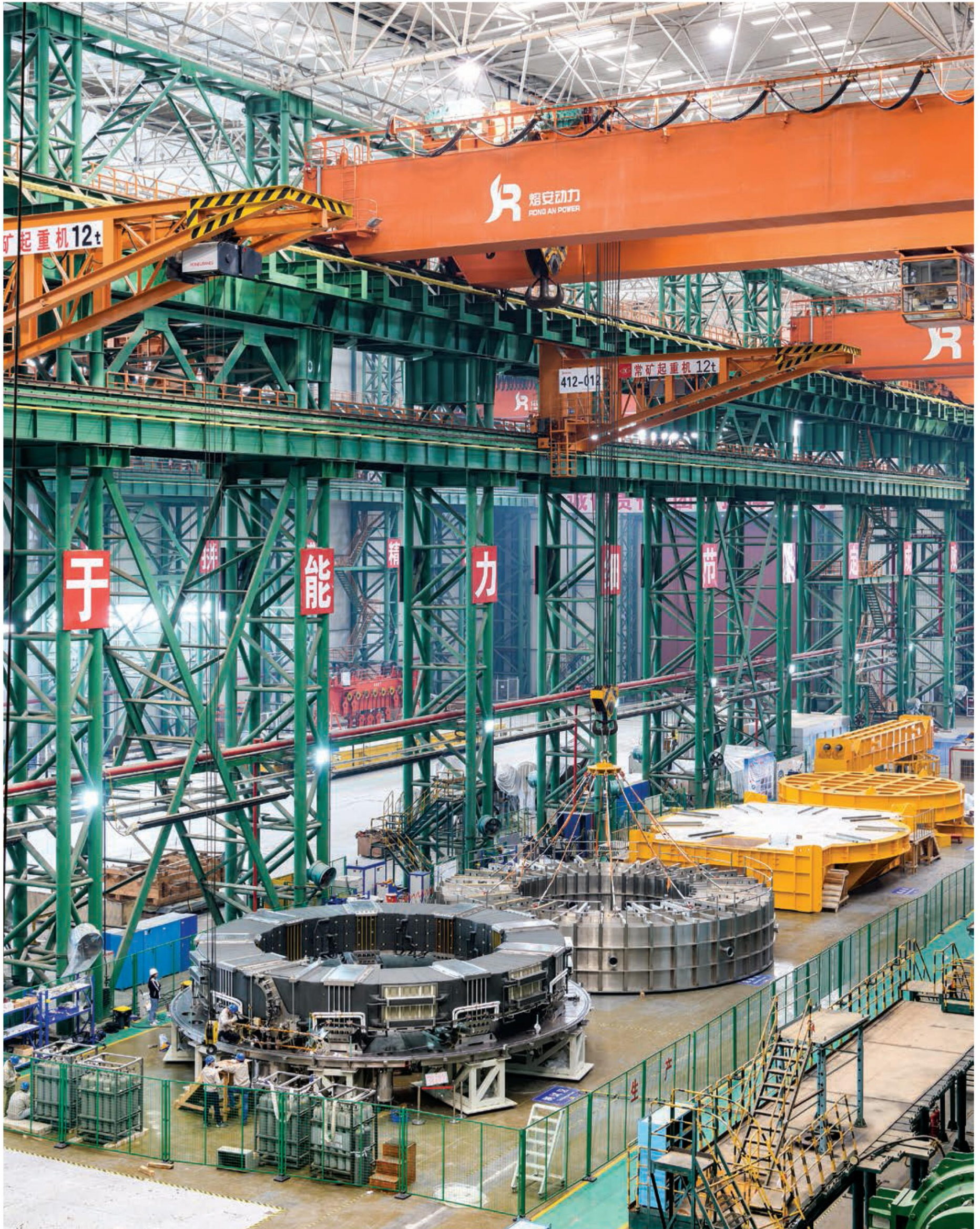
▲ PF6 being prepared for factory testing in Hefei. The heaviest of all the coils, it's scheduled to ship to France in December.
